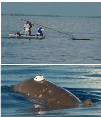
Top: Scientist deploy a DTag on a Blainville's beaked whale, using a flexible pole. Bottom: A DTag pictured on an adult female.
